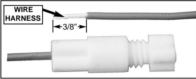
**NOTE:** If the strip length is too short, the connector will not function properly. The stripped portion of the wire must extend beyond the locking mechanism.
